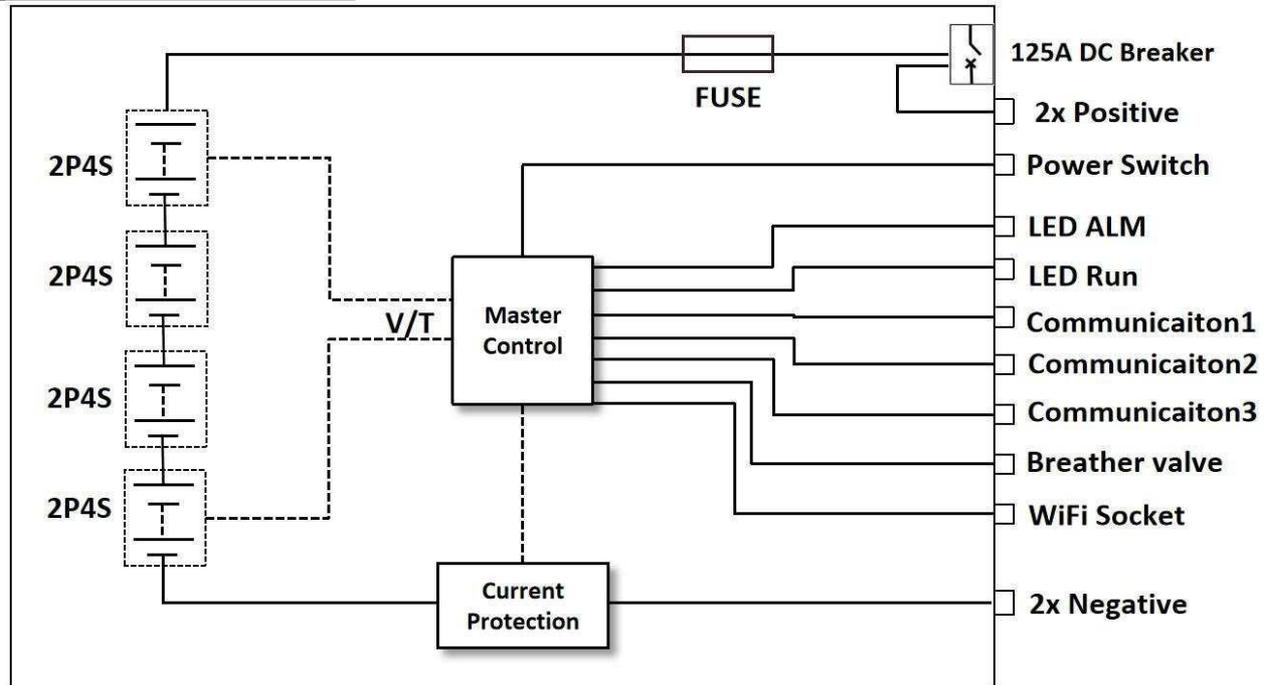
The product contains 32 lithium-ion cells in 2P16S connection, BMS PCB board, Fuse, DC breaker, MOSFET, Interconnecting wires and busbar.
