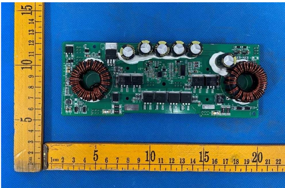
Figure 12. Front view of Current limit PCB Board
