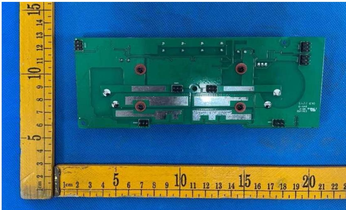
Figure 13. Back view of Current limit PCB Board
